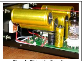
Figure 3. Fitting the Capacitors
