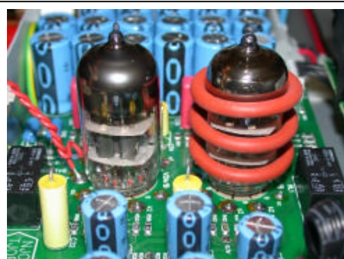
Figure 5. Tjoeb Ribs fitted to one of the valves
