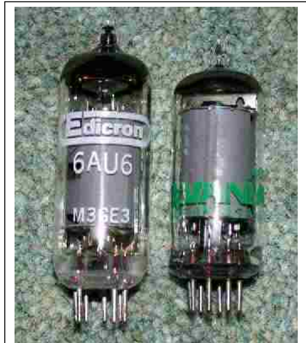
Figure 7. The Edicron 6AU6 with the Sylvania Equivalent 7543
