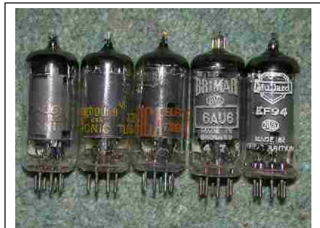
Figure 8. Other 6AU6s from Sylvania, Westinghouse, RCA, Brimar and the Mullard EF94
