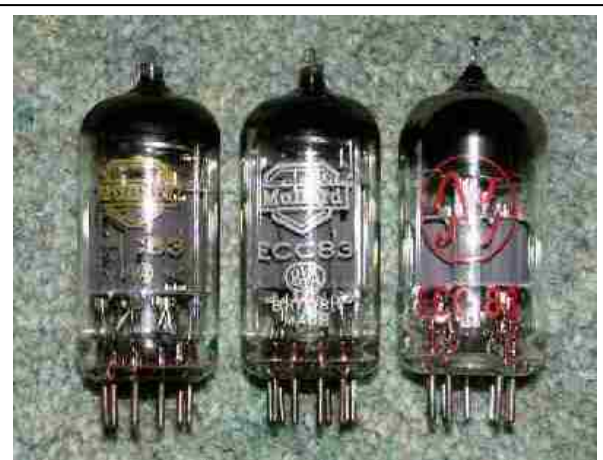
Figure 2. Three of the ECC83s: Mullard Yellow Logo, Mullard White Logo and JJ
