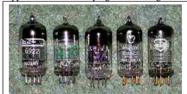
Figure 4. Some E88CC / 6922 Valves: Edicron, Philips, Russian Navigator, Mullard New Shield and Mullard Old Shield Logo
