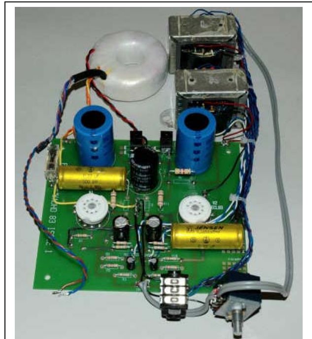
Figure 5. The Electronics Removed from the HD83
