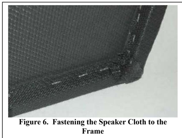
Figure 6. Fastening the Speaker Cloth to the Frame
