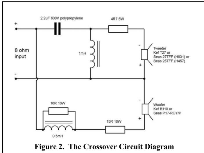
**Figure 2. The Crossover Circuit Diagram**
