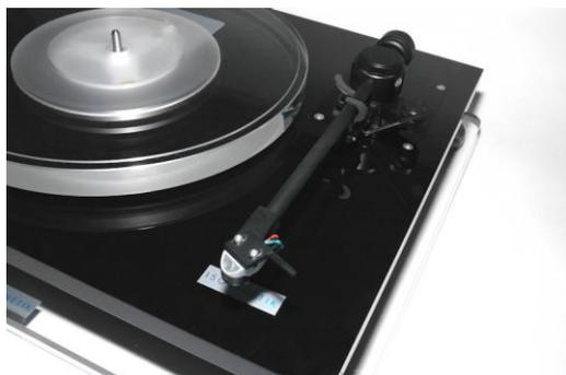
The plinth is CNC machined from highly polished billet acrylic, giving it a great finish. The feet are machined from Delrin and have dense sorbothane anti vibration pads. Incidentally, Delrin is an acetal resin and, according to the manufacturers (DuPont), it bridges the gap between metals and ordinary plastics with its unique combination of strength, hardness, resistance to solvents, low wear and low friction. The bearing assembly is made of phosphor-bronze and incorporates
