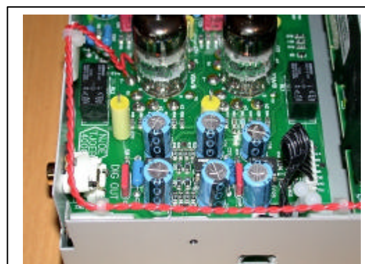
Figure 11. Wiring in the Power LED
