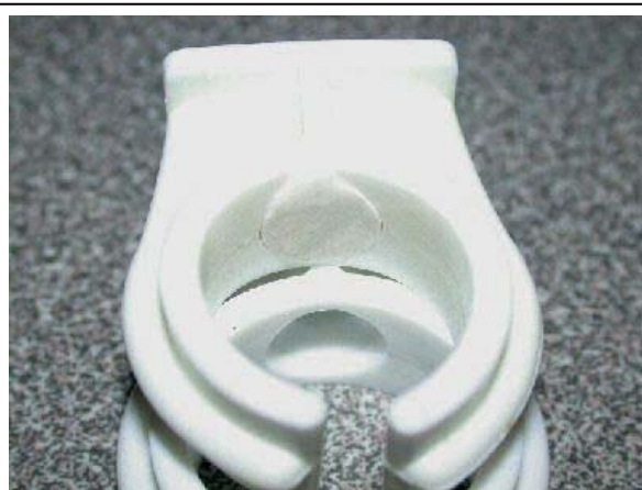
Figure 2. Plugging the Screw Hole with Modelling Compound
